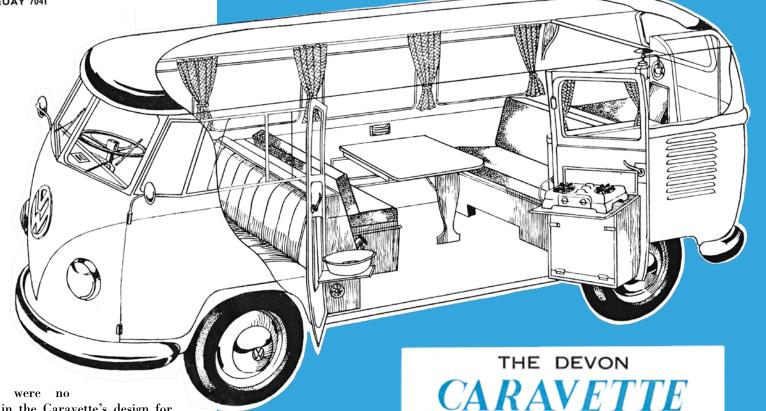
Although there were no major advances in the Caravette's design for or during 1960, the cooker was relocated onto the rear of the two-loading doors – as depicted in the enhanced brochure produced for that year. The company worded its latest sales material carefully, describing it as being 'arranged to provide indoor/outdoor cooking for use as required.'
